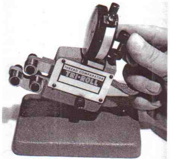
Setting the stop screw.
