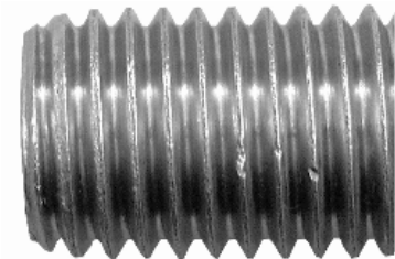
Minor thread nicking on external threads may still be found acceptable.
